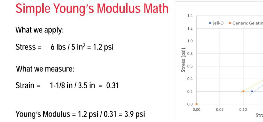
Multiple measurements can be graphed in a stress – strain diagram. The slope of the line past initial loading of the sample represents the Young's Modulus
