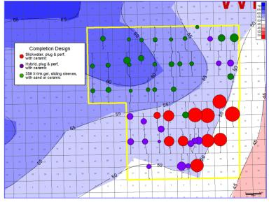
Middle Bakken wells just North of Williston. The three different bubble colors illustrate the dramatic difference in production performance for a design with a stout gel in sliding sleeve completions (in green); a hybrid design (in purple); and, the Liberty 2C's design (in red). While reservoir quality differences are minimal, the production response for the Liberty Design wells is 80 - 140% better.
