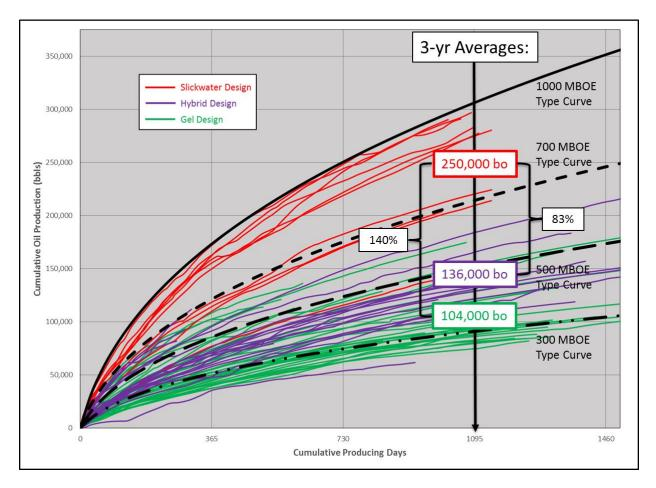
These three different completion designs also lead to dramatic differences in long-term production and ultimate recovery. EURs for the Liberty Design are much higher, tracking the 850 MBOE type curve, while the hybrid and gel designs track the 500 MBOE and the 300 MBOE type curves, respectively.
